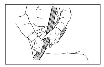
To unlatch the belt, just push the button on the buckle. When the safety belt is unbuckled or when the vehicle is turned off, the tension reducer will deactivate. The belt should go back out of the way.
